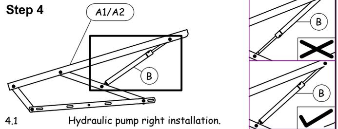
4.1 Hydraulic pump right installation.
